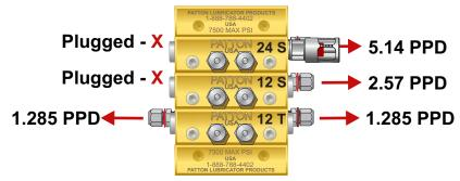
Step 2 Total divider block value is 48 & Cycle time is 28 seconds
