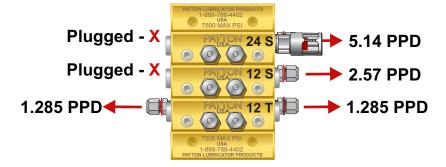
Step 1) Add the divider blocks together, = 48, & cycle time is 28 Seconds
