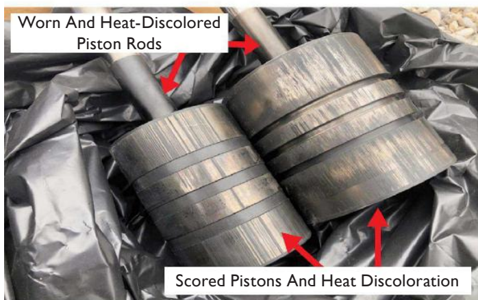
Figure 5. Scored Pistons, Worn Rods, Heat Discoloration On Rods
